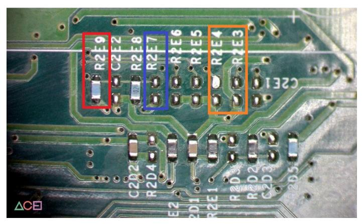
These adjustments should give you V1.45 at R1E1 going to the CPU CORE
